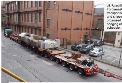
JB Rawcliffe & Sons Ltd successfully transported two castings from Sheffield Forgemasters International. The mill housings, destined for Venezuela, were transported from Sheffield to the Port of Goole where they where loaded to a barge and shipped to Duisburg Germany. JB Rawcliffe & Sons Ltd planned the route, organised the special orders, police and council liaison, street furniture removal and bridging of structures to successfully transport the castings without incident and on schedule.
